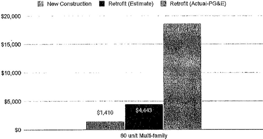
Fig 1: The least expensive time to install EV infrastructure is during new construction.<sup>1</sup>
